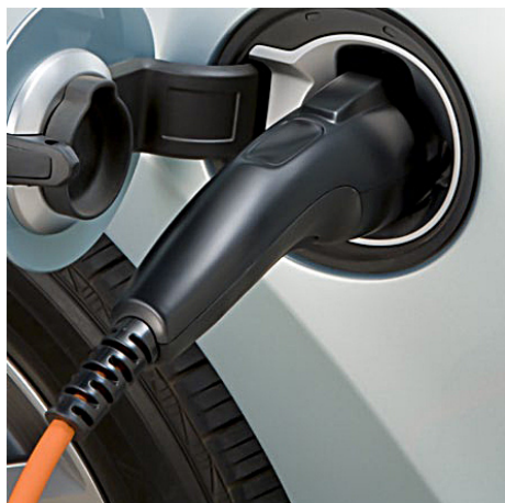
328 329 330 Figure 2.1 EV connector J1772™ Courtesy of General Motors 331
