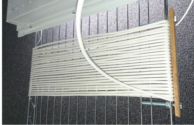
Figure 17. Example top view of bent cable.
